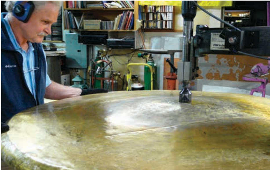
Our shrinking dies can shrink even the middle of large panels. Here Kent is shrinking bronze.
