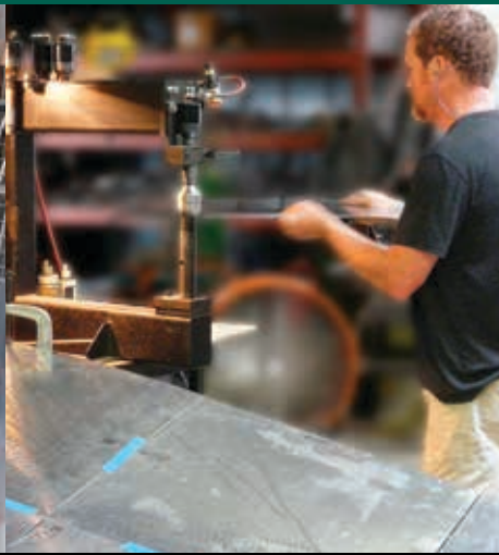
"Sky Wall," 12' x 60' public art installation, 180 panels of .060" 5052 alum. George Schroeder, San Antonio, TX. Center: George shaping panels with his TM hammer.
