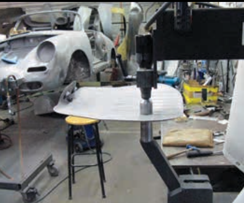
Porsche 911 (901) restoration. Dave DiMaria, Vintage Car Works, Englewood, CO. Far left: Making the new rear lid with his TM Model 2500 Air Power Hammer.
