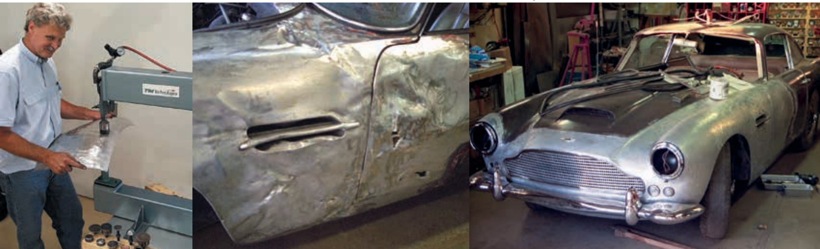
I to r — Prepping my first Hammers for Sun n' Fun, 1995; totaled Aston Martin DB4, before and after repairs done on my new Air Power Hammer, 1995.
