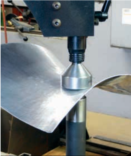
Saddle shape made using Reverse Dies
