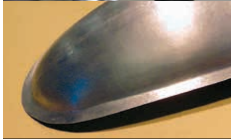
Flanged edges made using the Flanger Dies
