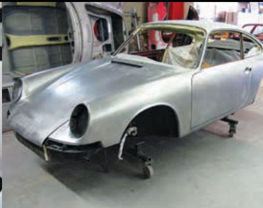
Porsche 911 (901) restoration. Dave DiMaria, Vintage Car Works, Englewood, CO. Far left: Making the new rear lid with his TM Model 2500 Air Power Hammer.
