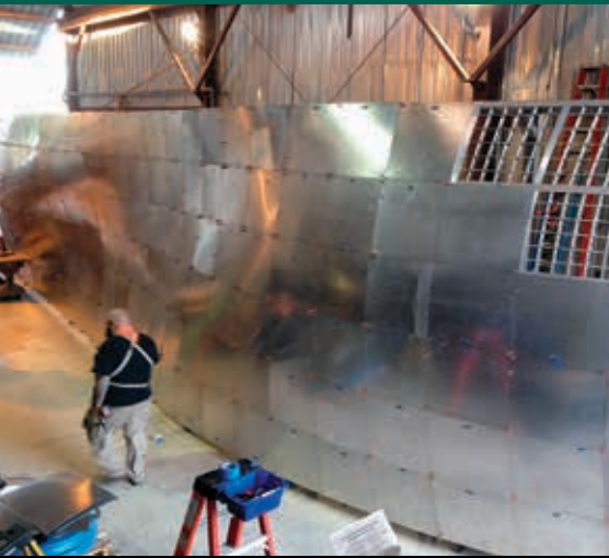
"Sky Wall," 12' x 60' public art installation, 180 panels of .060" 5052 alum. George Schroeder, San Antonio, TX. Center: George shaping panels with his TM hammer.
